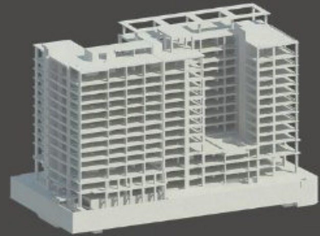
PART OF THE BIM STRUCTURAL MODEL
